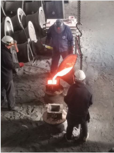
Casting a new bell.
