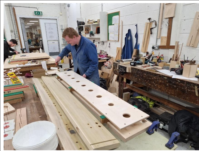
Pedal chest construction – preparing rackboards
