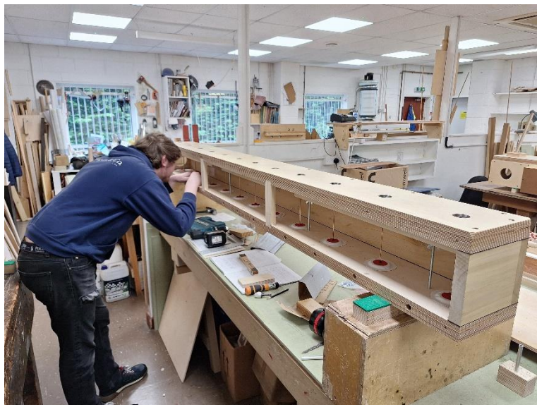
Pedal chest construction – setting up actions
