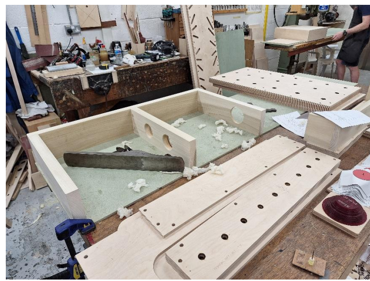
Pedal chest construction – assembling well and spine
