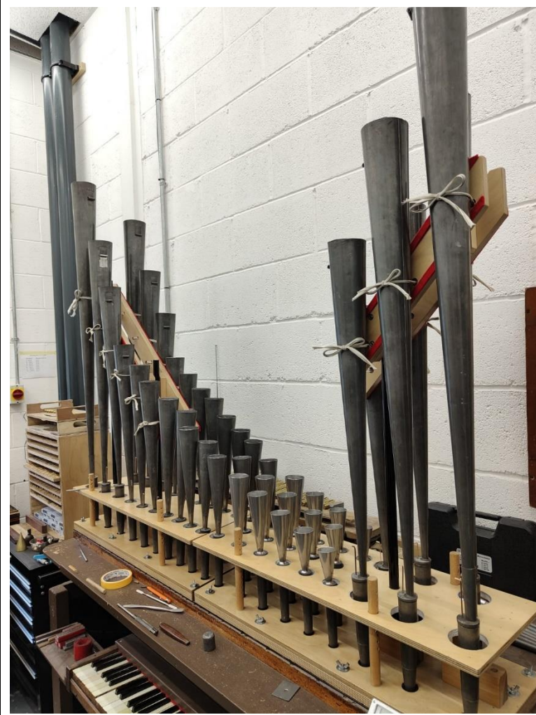
Swell Horn 8' on voicing machine
